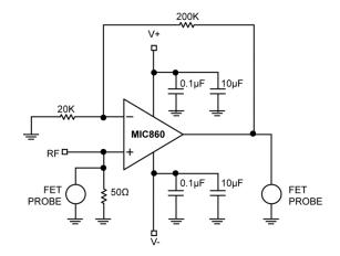
Test Circuit 1. A<sub>V</sub> = 10
