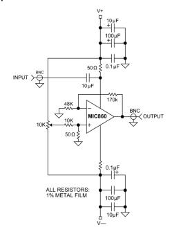
**Test Circuit 5. Positive Power Supply Rejection Ratio Measurement**
