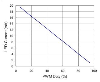
Figure 4. LED Current Variation with the PWM Dimming on FB
