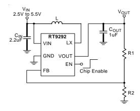
Figure 5. Application for Constant Output Voltage
