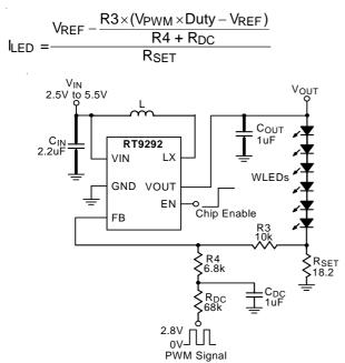
Figure 3. Filtered PWM Signal for LED Dimming Control of the RT9292
