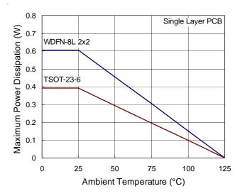
Figure 6. Derating Curves for RT9292 Packages
